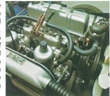
The Spitfire's distinguished 1493 cc engine is incredibly strict with its fuel-but enormously generous with its power. Developing 71 b.h.p. at 5,500 r.p.m. the sharp, confident acceleration can take you up to the 100 mph mark. And steady cruising at 50 mph can give you real economy, enhanced further by the optional overdrive—up to 50-6 miles to the gallon.\*
